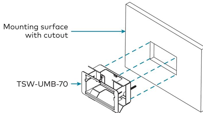
6. Reach into the assembly and push the rear half back so that it is behind the mounting surface completely. Ensure the front of the assembly is level.
