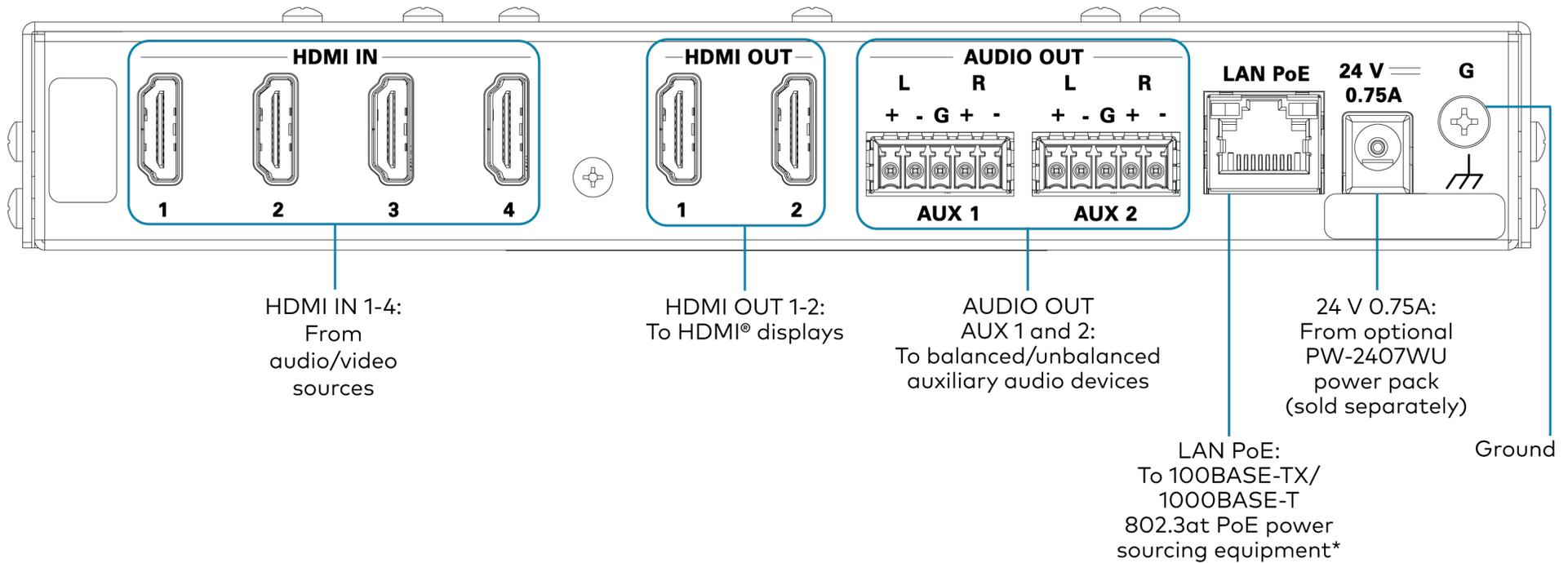
\*The LAN PoE port is a PoE PD (powered device) port. In order for the port to receive PoE, it must be connected to a PoE PSE (power sourcing equipment) port of a PoE switch. Wiring that connects to a PoE PSE port is designed for intrabuilding use only.
