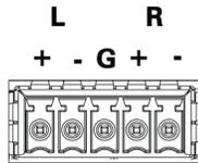
Refer to the following table and diagrams for analog audio output pin assignments and connection information.
