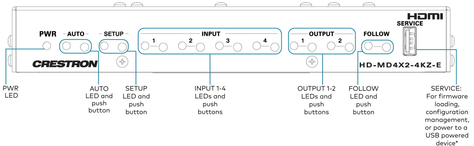
\*The SERVICE port can provide up to 5 V 500 mA power to a USB powered device.
